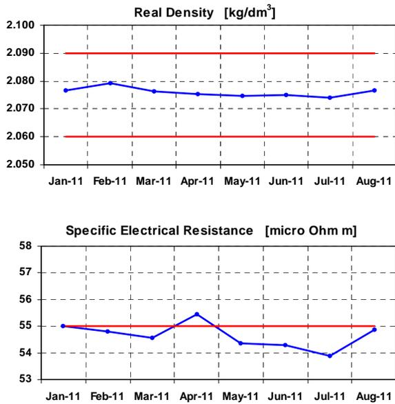
Figure 5: Real density and specific electrical resistance
