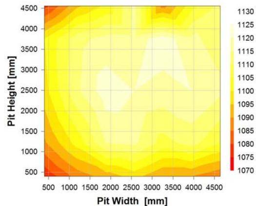
Figure 4: Real pit temperature distribution in °C
